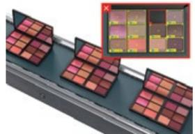
Missing-part Detection, QA/AC monitoring
